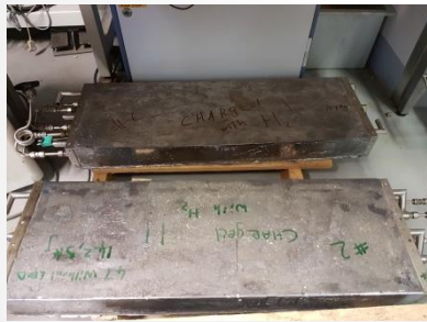
Left: two ready-to-use MH cassettes. Right: MH tank for forklift power module comprising 8 MH cassettes
