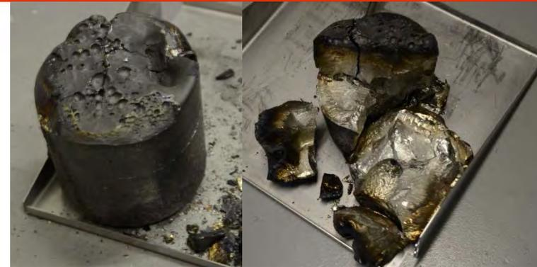
*Significant amounts of C and O in the impurity phases (casting in a graphite mould)*
