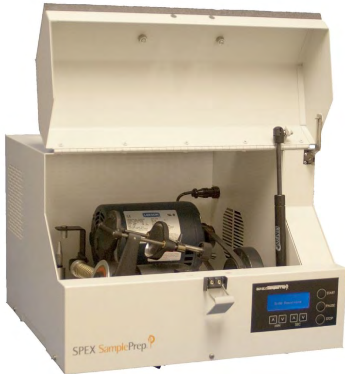
Spex mill: capacity ~5 g
